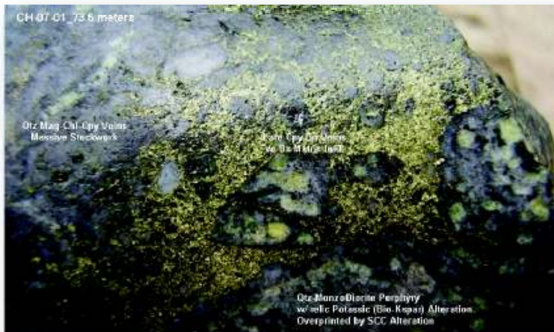
Photo 3. CH-07-01 73.5 meters: Stockwork veins (quartz+magnetite+hematite(specularite) veins and quartz+magnetite+chlorite+chalcopryrite veins) cutting quartz monzodiorite porphyry (weakly magnetic) with possible relic potassic (biotite-kspars) alteration of
