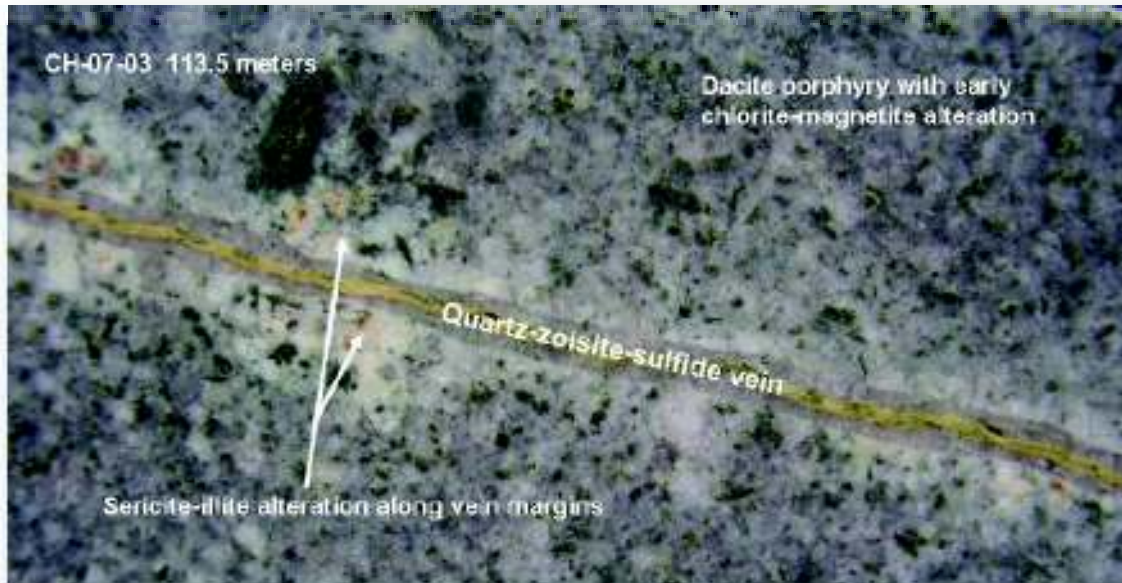
Photo 6. CH-07-03 113.5 meters: Porphyry-style sulfide mineralization associated with quartz stockwork veining (quartz+zoisite+sulfides) and sericite-illite alteration along the vein margin. Mineralization (chalcopyrite and pyrite) in veinlets is hosted in dacite porphyry.
