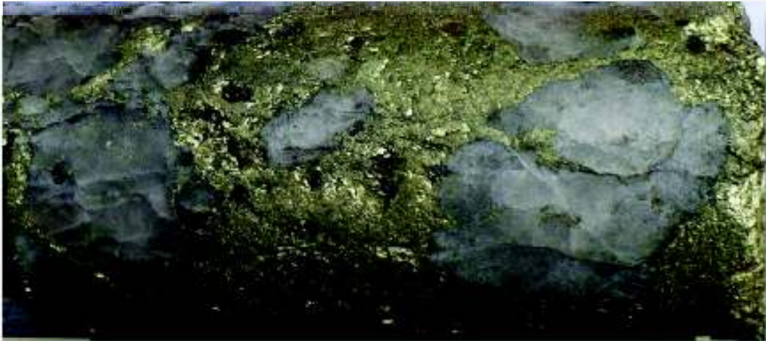
Photo 4. CH-07-03 238.1 meters: High grade (2.89% Cu, 0.25 g/t Au) copper-gold mineralization in this interval is hosted in quartz-magnetite stockwork veins and vein breccias. Mineralization is exclusively chalcopyrite, and occurs as veins and breccia infills.
